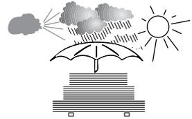
Avoid leaving the sheets in the rain, even if still wrapped, for extended periods, as water may condense inside the hollow core.
