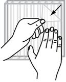
Remove the outer side or exterior protective film as soon as the installation of the whole glazed area is completed. This film should be removed shortly after installation. Failing to remove the film and exposing the film to direct sunlight may cause difficulties in removal due to deterioration of the film, and void the warranty.
